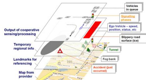
Fig. 1: The four layers of a LDM [1]
