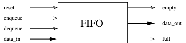
Figure 2: Hardware FIFO as black box. The clock signal is omitted.
